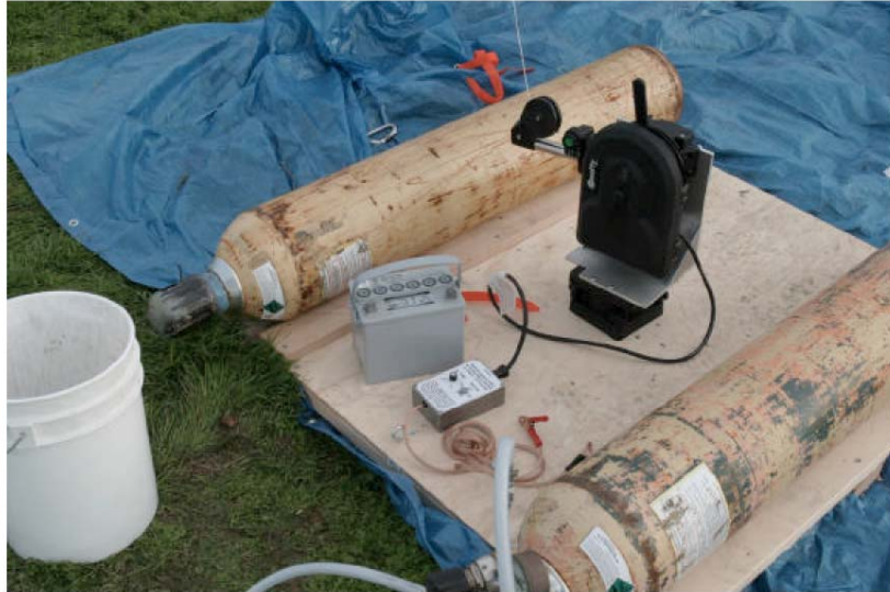
Figure 4 Winch Power Adapter, Battery Cables and Battery
